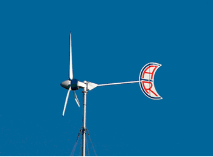
Fig. 1. ARE110 2.5KW grid-tied wind turbine on a 127ft ARE tilt-up tower in Newberg, Oregon. Designed, manufactured and installed by Abundant Renewable Energy
